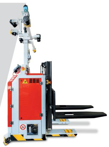
HIGH CAPACITY In relation to its reduced dimensions, the vehicle can move products loads up to 1.500 kg loads.
